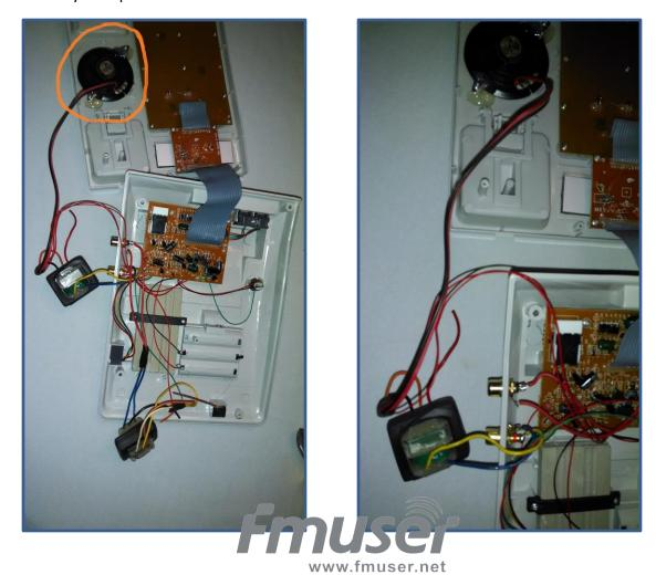
Here we connect a transformer, the transformer has two wires on one side and two on the other, two wires are for the voltage of 220 volts (110), which are normally red, and the two remaining, which are usually yellow, are cables that have 12 volts. on this occasion connect the red wires (220v or 100v), without regardless of position. The remaining two wires connected to a connector chassis RCA, mark as output audio.
