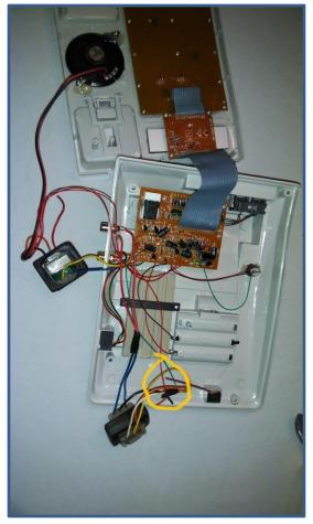
once we have identified the microphone, cut the wires and join the transformer, now will join the cables will be the 12 volt (yellow), regardless of the order, and blue (220 v or 110), connect them to the RCA connector chassis, which is unused, mark it as audio in.
